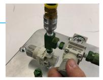
Attach plant air to "Compressed Air Inlet".
