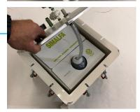
Release air pressure from cube using the "Fluid / Air Pressure Release Valve".
