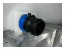
Connect the Kit | Camlock straight extender to the installed Camlock | 2" Female Buttress x 2" Part A Camlock 'Stubby', and lock in place with the locking arms of the camlock.
