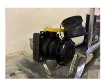
Remove valve safety cap and foil seal.
