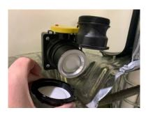
Cut zip tie holding male camlock attachement and thread onto the tote valve.
