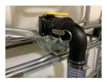
Turn valve lever clockwise to open.
