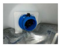
Connect the Camlock | 2" Female Buttress x 2" Part A Camlock 'Stubby' to the tote valve. WARNING – Do not touch internal valve components as opening of the valve may occur.
