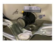
Connect the female camlock that is currently attached to the 2" PVC hose to the male camlock on tote valve and lock in place with the locking arms of the camlock.
