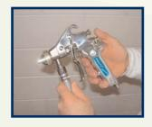
1. Attach the spray gun to stainless steel fitting on Free Flowing hose.
