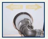
3. Connect the female camlock that's currently attached to the 2" PVC hose to the male camlock adaptor already on the tote and lock in place with the locking arms of the Camlock.
