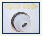
2. Remove valve safety cap and connect the male camlock adaptor.
